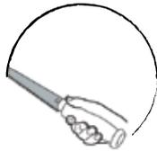
If the cable has not yet been run, do so now that you have better access to the ceiling. Once the speaker cable has been run, pull the end of the cable out of the speaker cut-out, strip back a section of the jacket as needed, and then expose 1/2" (13mm) of each conductor.
